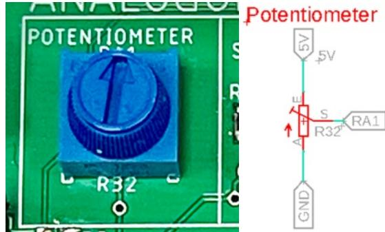
When read by the ADC on the PIC, the value will range from 0-1023. This can be converted into 0-100% by multiplying the ADC result by 0.098.
