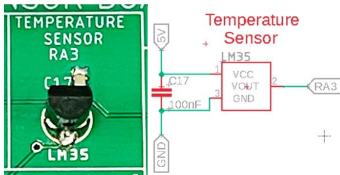
When read by the ADC on the PIC, the value will range from 0-1023. This can be converted into Centigrade by multiplying the ADC result by 0.489
