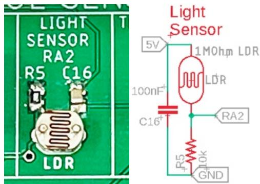
When read by the ADC on the PIC, the value will range from 0-1023. This can be converted into 0-100% by multiplying the ADC result by 0.098.
